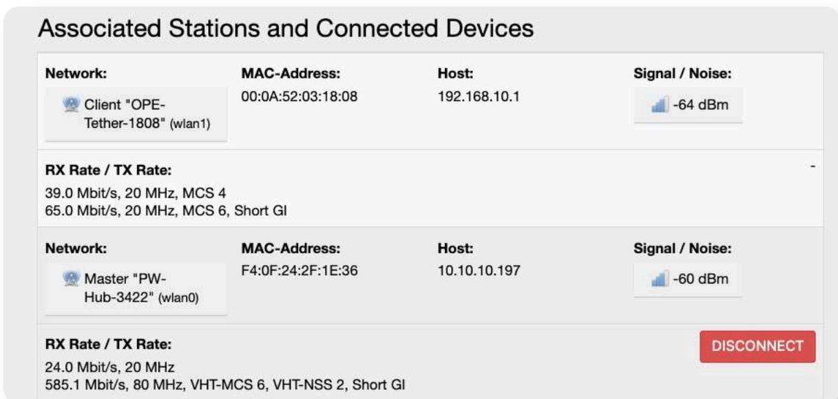
You will see the SSID of the remote station listed with signal strength and a transmit (TX) and receive (RX) rate. You will know that the station is not available, or you were not successful (if say you entered the password incorrectly) when the signal bounces between 0 and some value and the RX/TX rates drop to zero.
